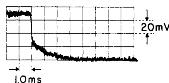
FIG. 2.—Oscillograph trace of a mixture of malate dehydrogenase with DPNH, both in equal amounts at 6 \mu\text{M} in phosphate, pH 7.0, ionic strength 0.1. Electronic RC filter set at 0.95 \mu\text{sec} , horizontal deflection 1.0 \text{ msec/cm} , vertical deflection 20 \text{ mv/cm} .
